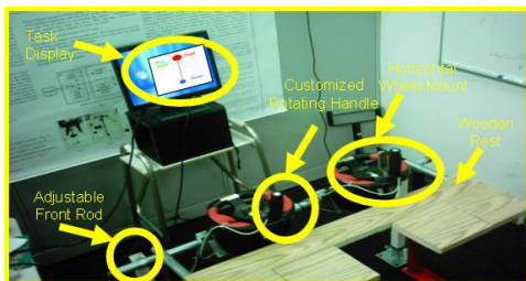
Figure 7. Bilateral mode with a de-coupled wheel setting. Two wheels were used for tracking.
