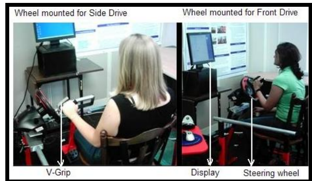
Figure 1. TheraDrive System: The wheel can be used in front and side driving, For this study, the wheel will be used in front driving mode.
